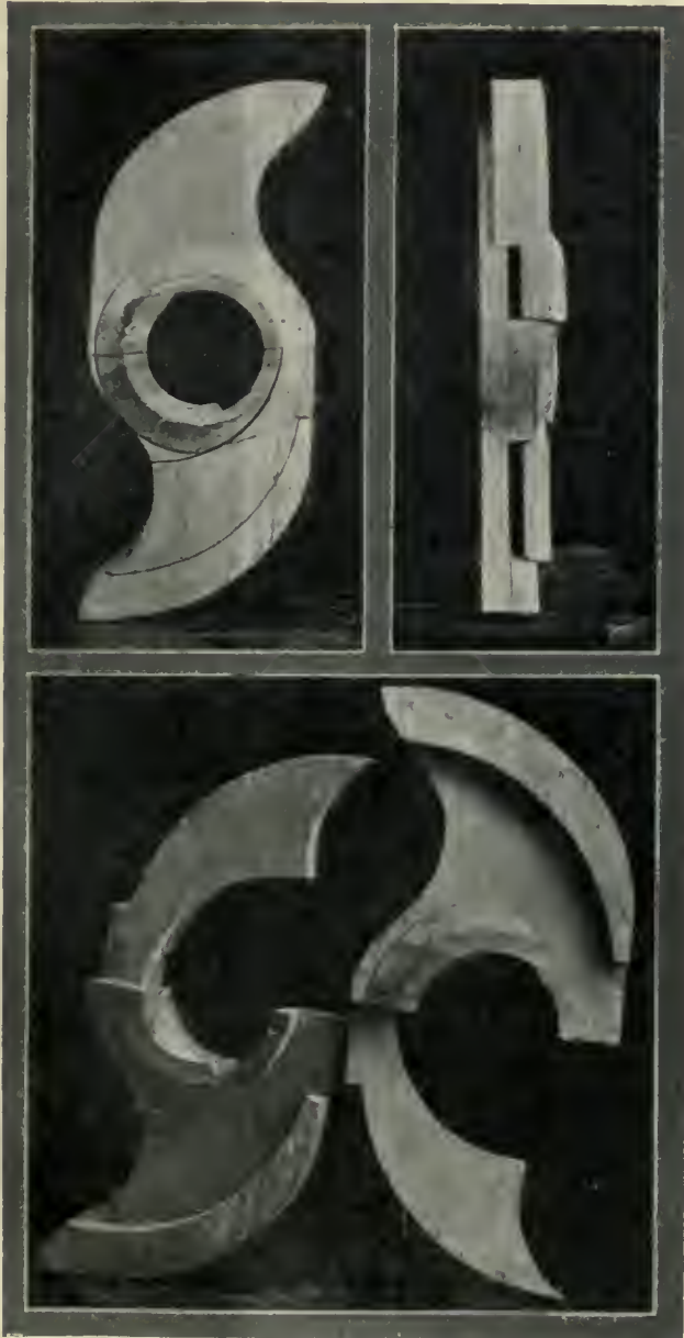
SHOWING WOODEN MODEL OF CAM. (1) COMPLETE CAM; (2) FITTING CAM TOGETHER; (3) CAM IN HALVES, SHOWING CONSTRUCTION.
